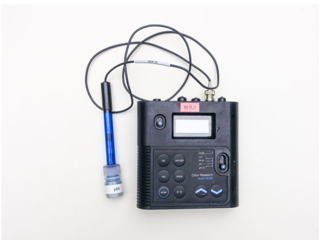
Abb. 41: pH-Meter (Orion Research, Modell SA 250)
